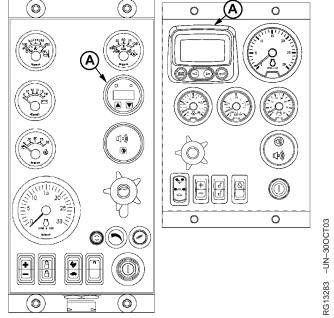
Hour Meter On Earlier Panel (Left) or Later Panel (Right) (Except 4.5 L "270" Engines)
