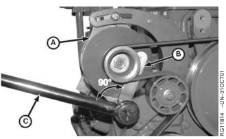
Belt Tension Tool and Torque Wrench
