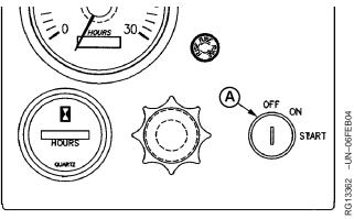
Key Switch on Instrument Panel (Later Engines)
