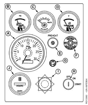
Instrument Panel and Gauges (Later 4.5 L "270" Engines)
