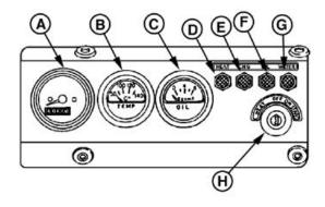
Instrument Panel and Gauges (4.5 L "270" Engines)
