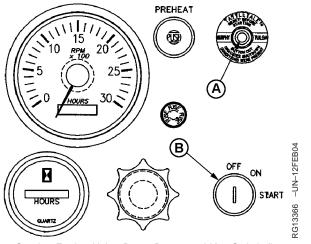
Starting Engine Using Reset Button and Key Switch (Later Engines)
