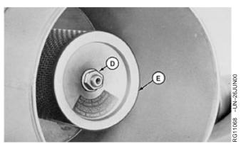
Retaining Nut and Secondary Element
