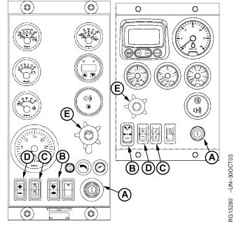
Start And Idle Engine On Earlier Panel (Left) or Later Panel (Right)
