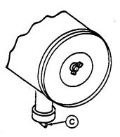
Dust Unloader Valve and Restriction Indicator
