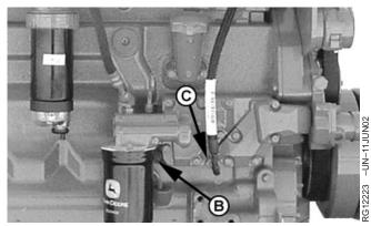
Engine Block Coolant Drain Plug- 475 Engines
