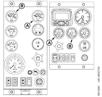
Oil Pressure and Coolant Temperature Gauges On Earlier Panel (Left) or Later Panel (Right)
