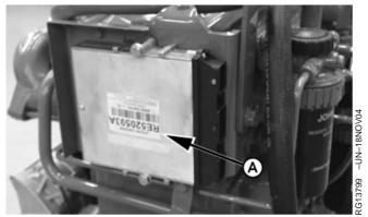
Record Engine Control Unit (ECU) Serial Number
