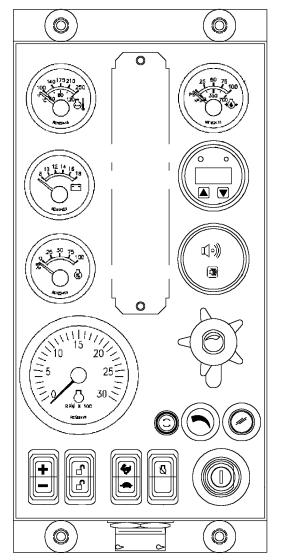
Instrument Panel For Earlier Electronically Controlled Engines (See Section 16)
