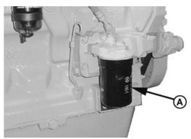
Oil Filter And Mounting Header
