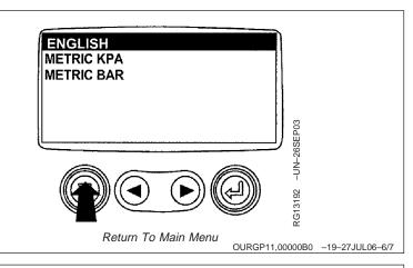
7. Press the "Menu" key to return to the engine parameter display.
