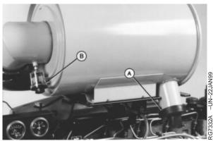
Dust Unloader Valve and Indicator Gauge
