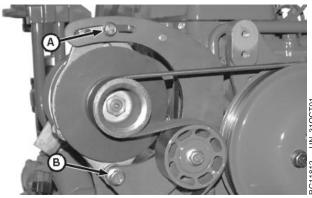
Alternator Bracket and Cap Screws
