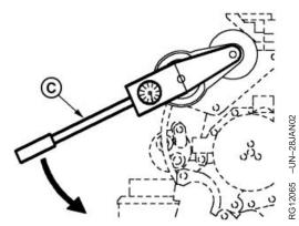
Align Torque Wrench With Pulley and Tensioner
