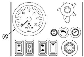
Using Tachometer to Check Engine Speeds
