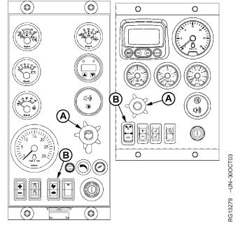
Analog Throttle Control and Speed Select Switch On Earlier Panel (Left) or Later Panel (Right)
