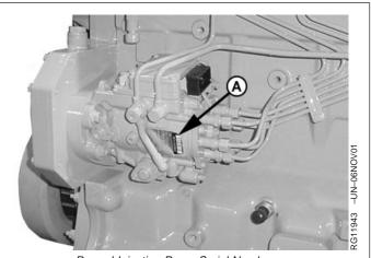
Record Injection Pump Serial Number
