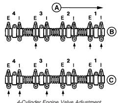
4-Cylinder Engine Valve Adjustment
