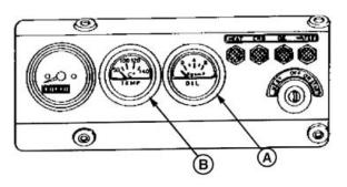
Oil Pressure and Coolant Temperature Gauges (Earlier Engines)
