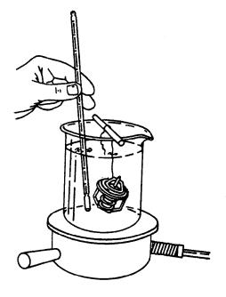
Testing Thermostat Opening Temperature
