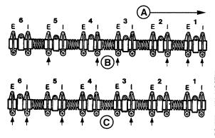
6-Cylinder Engine Valve Adjustment
