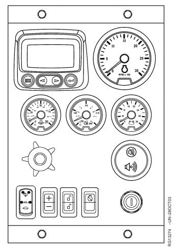
Full-Featured Instrument Panel For Later Electronically Controlled Engines (See Section 17)
