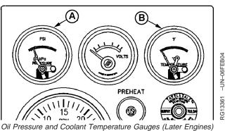
A—Oil Pressure Gauge **B**—Coolant Temperature Gauge -UN-17FEB03
