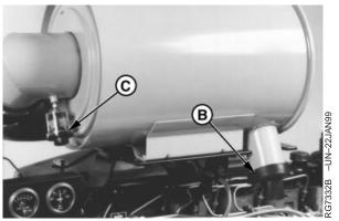
Underloader Valve and Air Restriction Indicator
