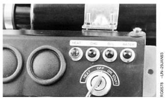
Key Switch in "ON" Position (4.5 L "270" Engines)
