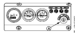
Key Switch on Instrument Panel (Earlier Engines)
