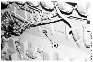
Engine Block Drain Valve- Except 475 Engines
