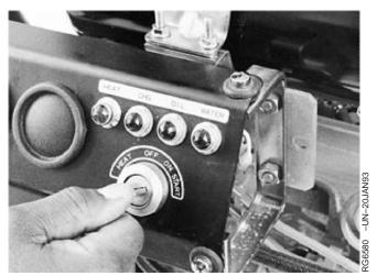
Starting Engine Using Key Switch (Earlier Engines)
