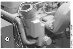
Thermostat Cover-to-Coolant Pump Tube
