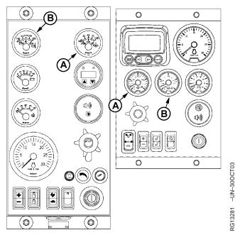
Watch Coolant Temperature and Oil Pressure On Earlier Panel (Left) or Later Panel (Right)
