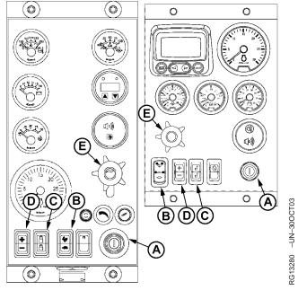
Stopping the Engine On Earlier Panel (Left) or Later Panel (Right)
