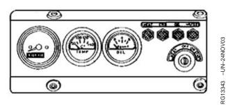
Instrument Panel For Earlier Mechanically Controlled "270" Engines (See Section 18)
