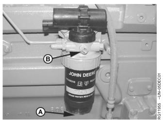
Drain Primary Fuel Filter (If Equipped)
