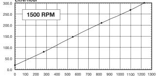
Gross Engine Power Output - kWm (U.S. Gal = Litres x 0.2642) (BHP = kWm x 1.34)
